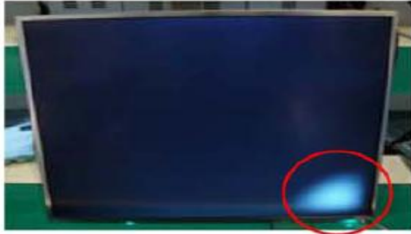
Panel Mura, Light leakage
