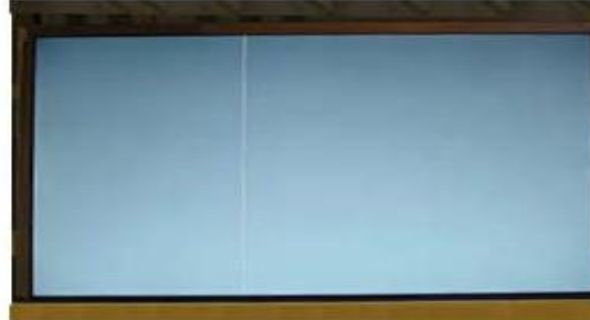
Vertical Line Source TAB IC Defect
