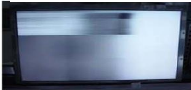
Horizontal Block Gate TAB IC Defect
