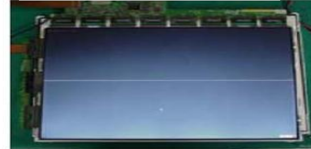
Horizontal line Gate TAB IC Defect
