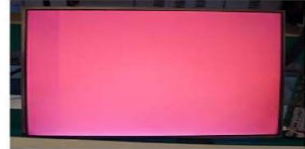
Vertical Block Source TAB IC Defect
