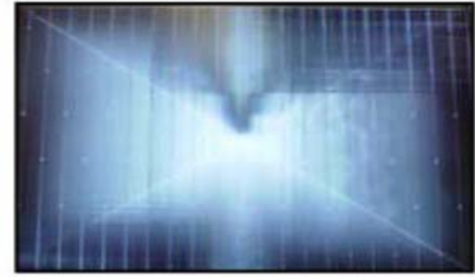
Solder defect, Short/Crack
