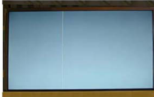
Vertical Line Source TAB IC Defect
