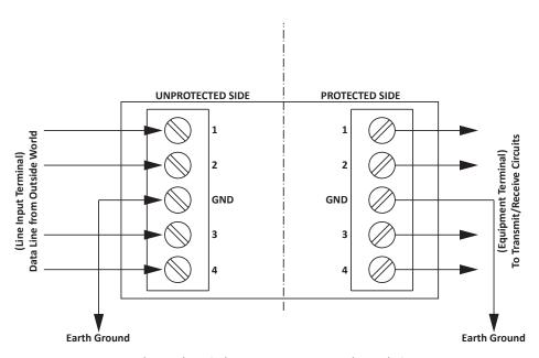
**Note:** Both ground terminals are common. Use second ground wire to reduce impedance on long runs to earth ground connections.
