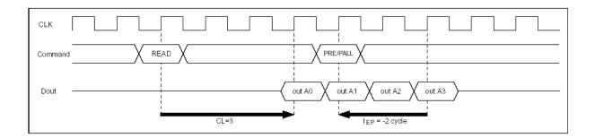
Recharge command Interval (same bank): To stop output data
