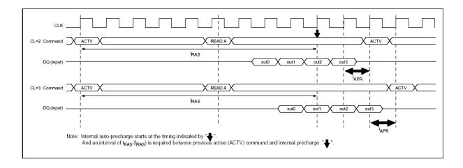
**Write with auto-precharge:** In this operation, since precharge is automatically preformed after completing a burst write or single write operation, a precharge command need not be executed after each write operation. The command executed for the same bank after the execution of this command must be the bank active (ACTV) command. In addition, an interval of I<sub>APW</sub> is required between the final valid data input and input of next command.
