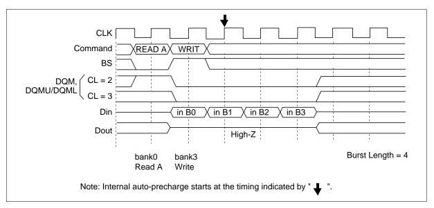
**2. Same bank:** The consecutive write command from read with auto precharge (the same bank) is illegal. It is necessary to separate the two commands with a bank active command.
