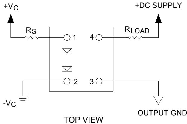
Figure 2. Terminal Connections
