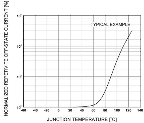
Figure 10. Repetitive Peak Off-state Current vs Junction Temperature
