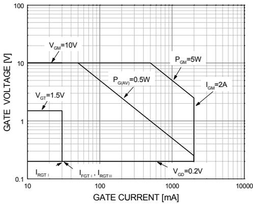
Figure 3. Gate Characteristics
