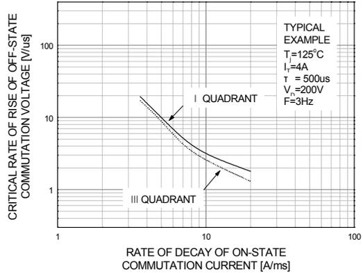
Figure 16. Commutation Characteristics
