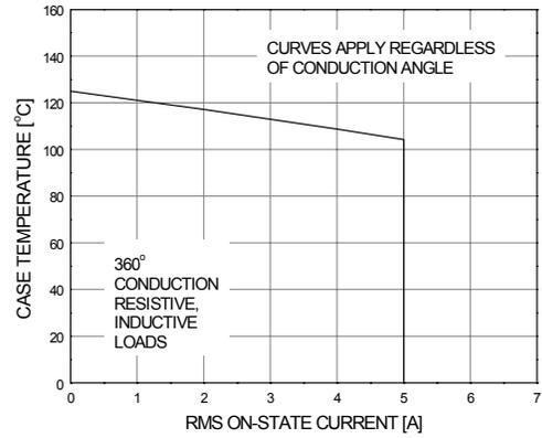
Figure 8. Allowable Case Temperature vs Rms On-state Current
