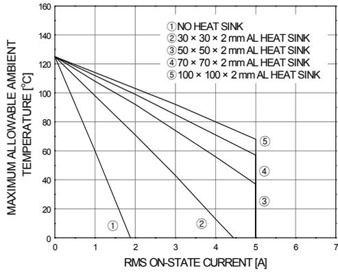
Figure 7. Allowable Ambient Temperature vs Rms On-state Current
