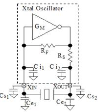
You can write the following equations for the total capacitance at each crystal pin:
