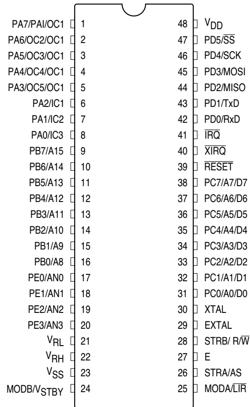
Figure 3 48-Pin DIP Pin Assignments
