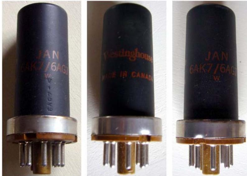
6AK7 is one of the very few tubes registered in US by Canadian REL. Through WWII Research Enterprise Limited was the engineering and manufacturing arm of Canadian National Research Council, established to build optical devices, as binoculars and gunsights, and radar sets.
