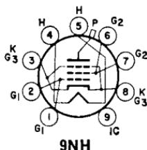
Magnoval type used as horizontal-deflection amplifier in television receivers. Outlines section, 35B; requires neonoval 9-contact socket. Typical instantaneous characteristics (measured with recurrent waveform such that maximum ratings are not exceeded): plate volts, 75; grid-No.2 volts, 200; grid-No.1 volts, -10; plate mA, 440; grid-No.2 mA, 37. Types 13GB5/XL500, 18GB5/LL500 and 27GB5/PL500 are identical with type 6GB5/EL500 except for heater ratings.
