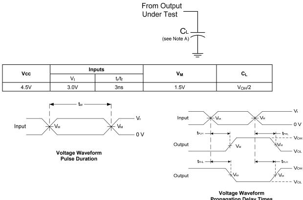
Propagation Delay Times Inverting and Non Inverting Outputs
