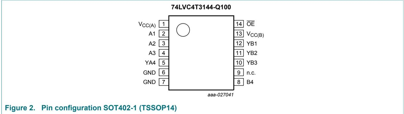
Figure 2. Pin configuration SOT402-1 (TSSOP14)
