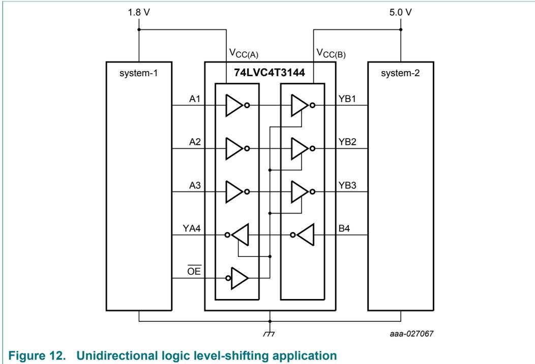
Figure 12. Unidirectional logic level-shifting application
