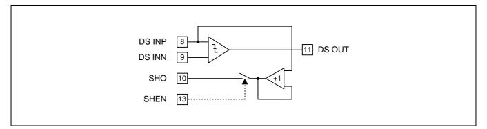
The output of the data slicer (DS-OUT) is a CMOS compatible bitstream. However, it is recommeded that an external NPN amplifier stage be used to drive the CMOS baseband processor, in order to minimize the amount of ground and supply currents in the S1T8531 which might desensitize the chip.
