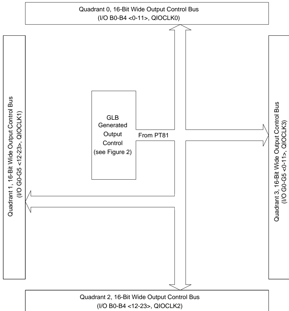
Figure 5. Output Control Bus and Quadrant Organization
