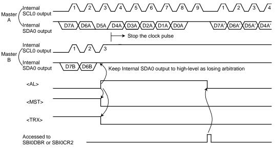
Figure 3.10.20 Example of a Master Device B (D7A = D7B, D6A = D6B)
