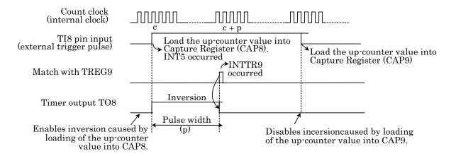
Figure 3.8.13 One-shot pulse output (without delay)
