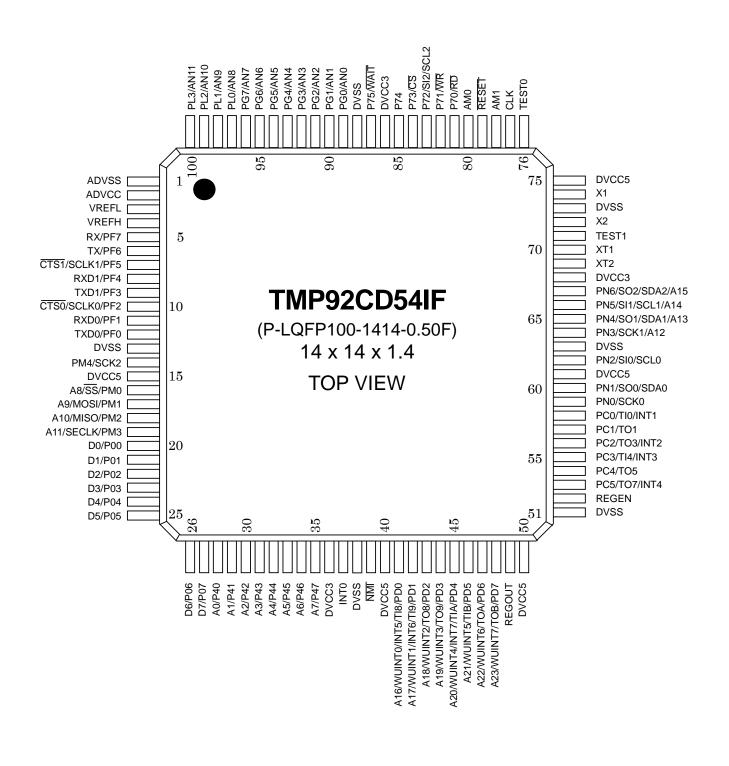
Figure 2.1 TMP92CD54I Pin Assignment
