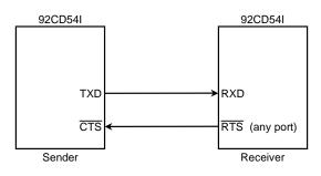
Figure 3.9.6 Handshake function
