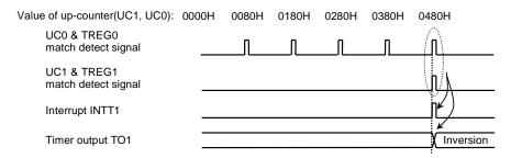
Figure 3.7.20 Timer output by 16-Bit Interval Timer Mode
