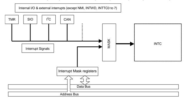
Figure 3.4.4 Block Diagram of Interrupt Mask Control
