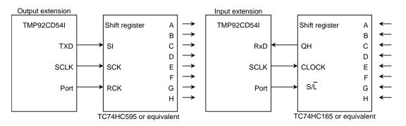
Figure 3.9.18 Example of SCLK Output Mode Connection
