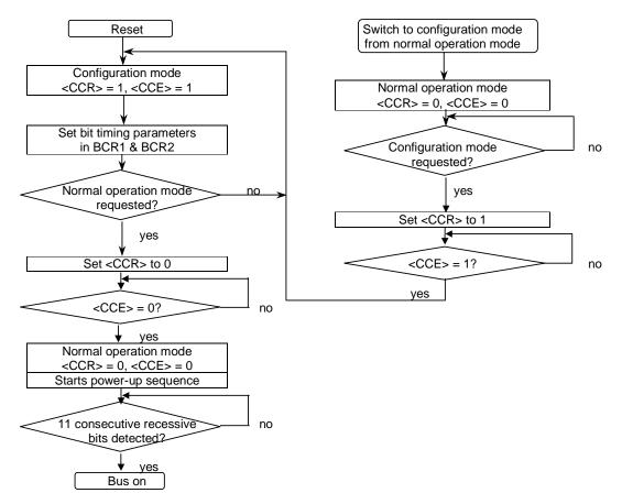
Figure 3.12.5 Flowchart of CAN Initialization
