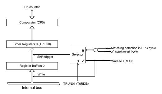
Figure 3.7.6 Configuration of TREG0
