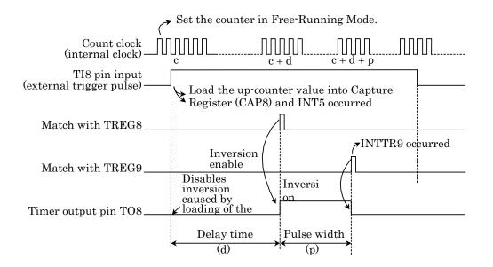
Figure 3.8.12 One-shot pulse output (with delay)
