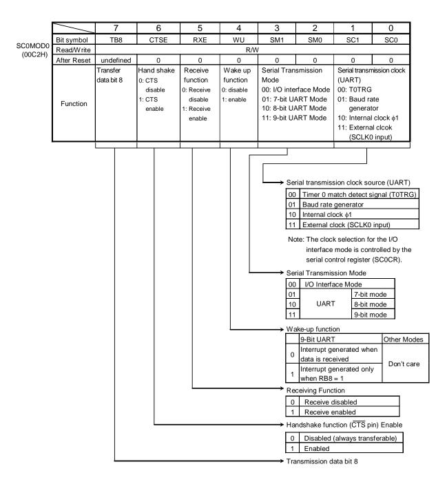
Figure 3.9.8 Serial Mode Control Register (channel 0, SC0MOD0)
