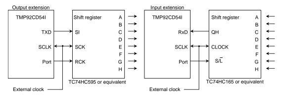
Figure 3.9.19 Example of SCLK Input Mode Connection
