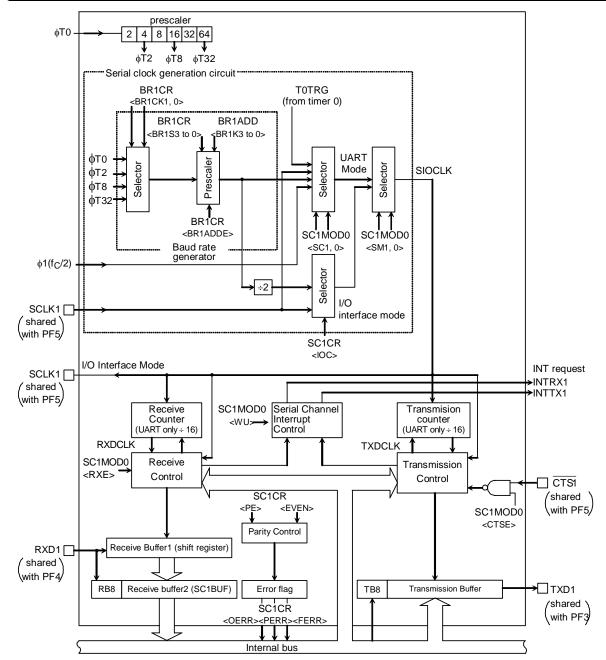
Figure 3.9.3 Block diagram of the Serial Channel 1
