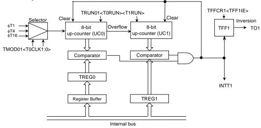
Figure 3.7.19 Block diagram of 16-Bit interval timer Mode
