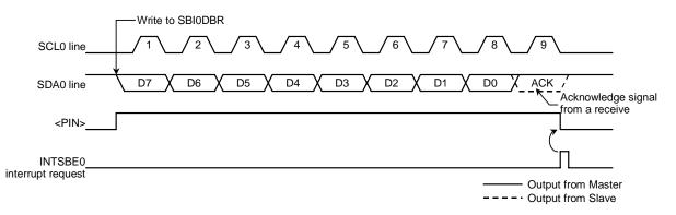
Figure 3.10.22 Example in which <BC2 to 0> = "000" and <ACK> = "1" in Transmitter Mode
