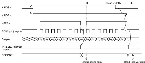
Figure 3.10.41 Receiver Mode (example: Internal clock)
