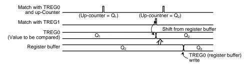
Figure 3.7.23 Operation of register buffer
