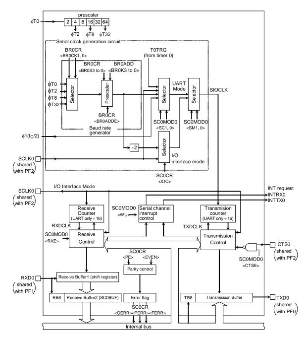
Figure 3.9.2 Block diagram of the Serial Channel 0
