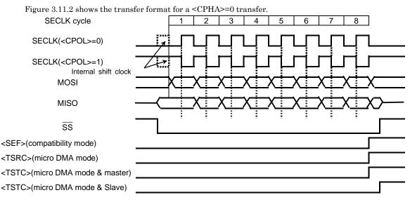
Figure 3.11.2 Transfer Format of <CPHA>=0
