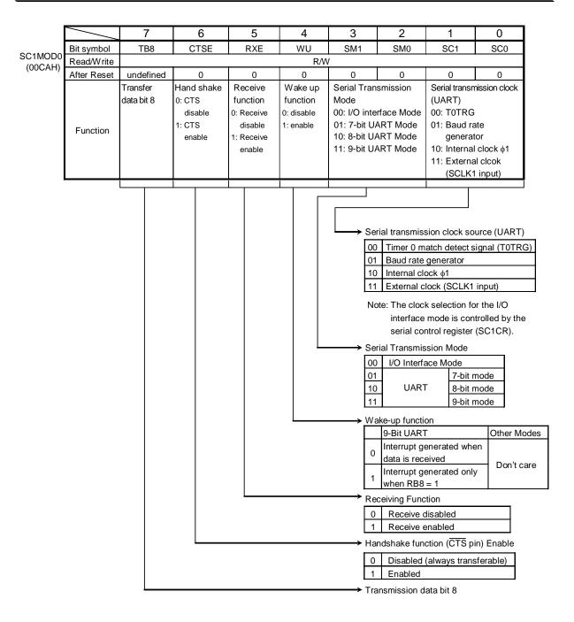
Figure 3.9.9 Serial Mode Control Register (channel 1, SC1MOD0)
