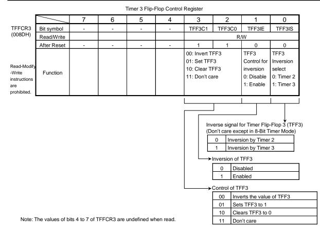
Figure 3.7.14 Register for 8-bit Timers
