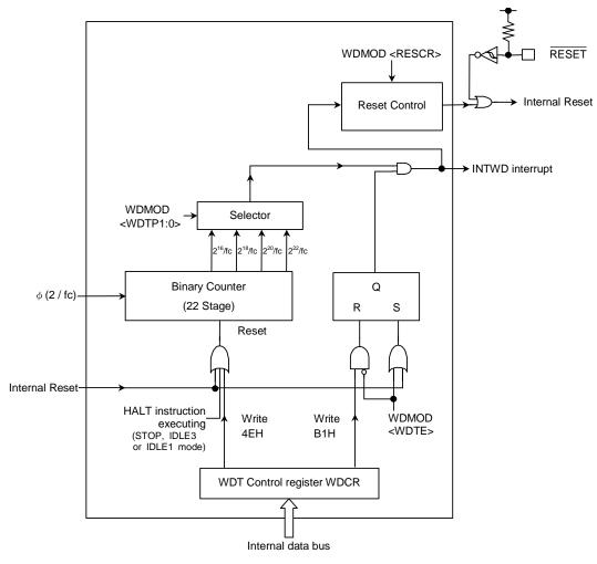
Figure 3.14.1 Block Diagram of Watchdog Timer
