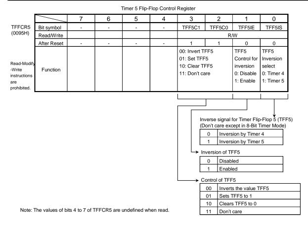
Figure 3.7.15 Register for 8-bit Timers
