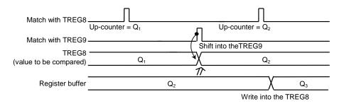
Figure 3.8.10 Operation of Register Buffer
