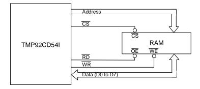
Figure 3.6.1 Example of connecting external memory (external RAM)
