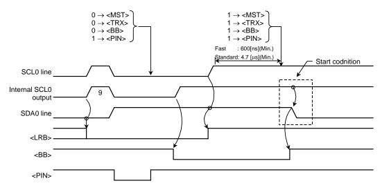
Figure 3.10.26 Timing Diagram when Restarting
