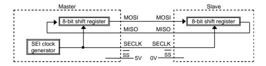
Figure 3.11.4 Connection between Master and Slave in SEI
