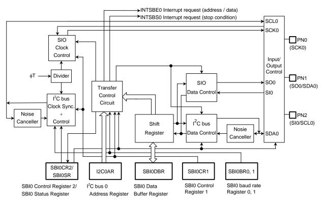
Figure 3.10.1 Serial Bus Interface 0 (SBI0)
