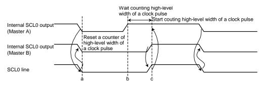
Figure 3.10.16 Clock Synchronization
