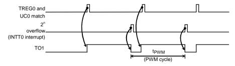
Figure 3.7.24 8-bit PWM waveforms
