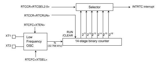
Figure 3.16.1 Block diagram for timer for real-time clock
