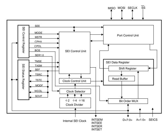
Figure 3.11.1 SEI Block Diagram
