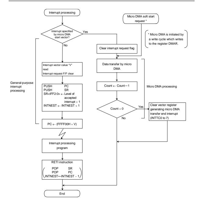
Figure 3.4.1 Interrupt and micro DMA processing sequence
