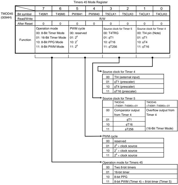
Note : When setting the TI4 pin, first set the Port C setting, then TMOD45.
