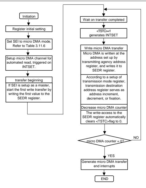
Figure 3.11.8 Flowchart for Micro DMA Write only Transfer
