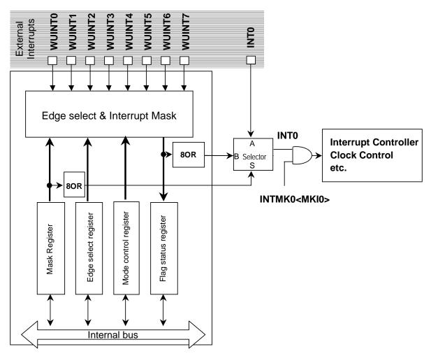
Figure 3.4.5 Block diagram of ON/OFF logic
