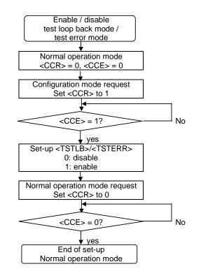
Figure 3.12.6 Flowchart of the test loop back mode / the test error mode set-up
