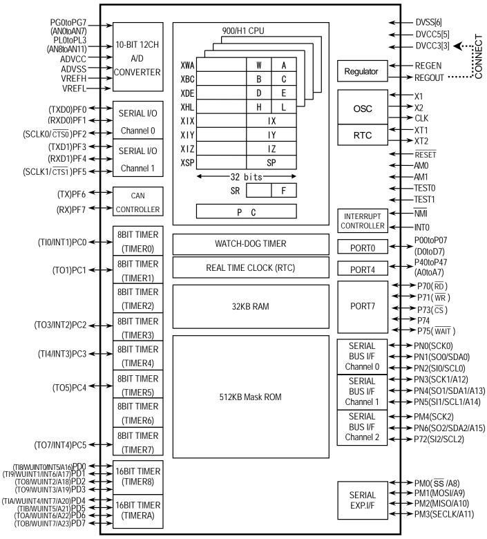
Figure 1 TMP92CD54I block diagram
