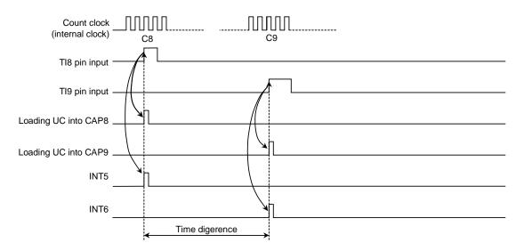
Figure 3.8.16 Time difference measurement
