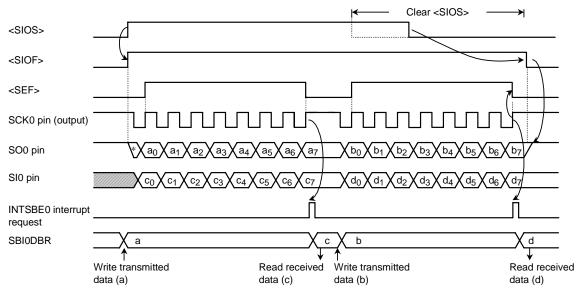
Figure 3.10.42 Transmit/Received Mode (Example : Internal clock)
