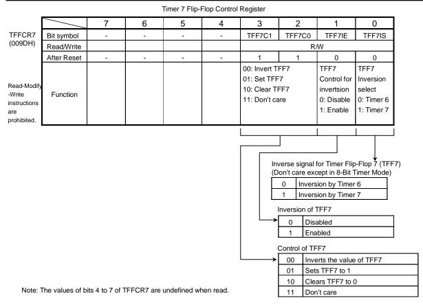
Figure 3.7.16 Register for 8-bit Timers
