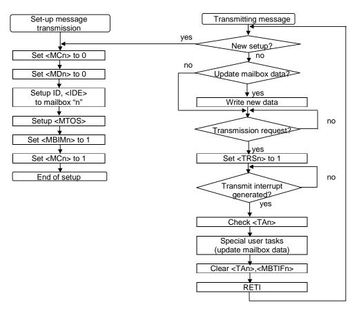
Figure 3.12.7 Flowchart of message transmission (Example)
