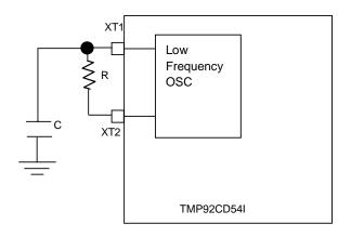
Figure 3.16.3 A external circuit for CR oscillation
