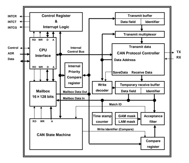
Figure 3.12.1 Block Diagram of CAN Controller
