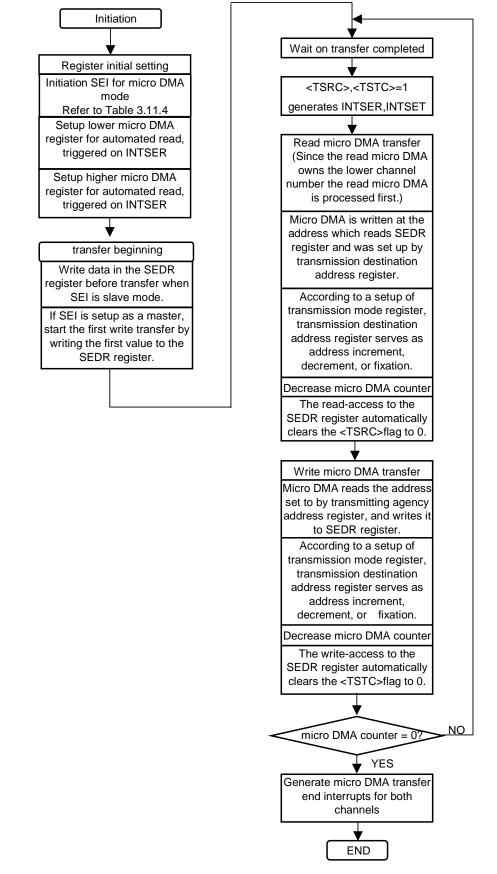
Figure 3.11.6 Flowchart for Micro DMA Read/Write Transfer
