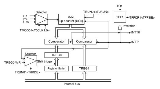
Figure 3.7.22 Block diagram of 8-Bit PPG Output Mode
