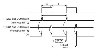
Figure 3.7.21 8 bit PPG output waveforms
