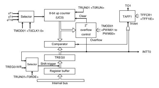
Figure 3.7.25 Block diagram of 8-Bit PWM Mode
