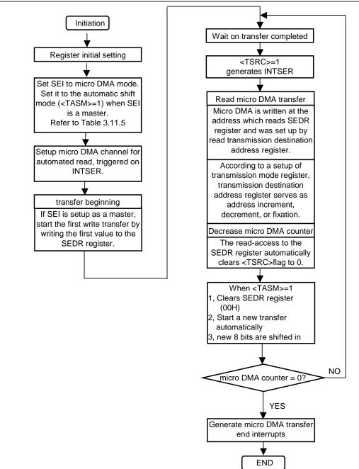
Figure 3.11.7 Flowchart for Micro DMA Read only Transfer
