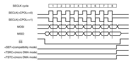
Figure 3.11.3 Transfer Format of <CPHA>=1
