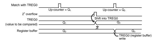
Figure 3.7.26 Register buffer operation
