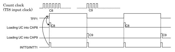
Figure 3.8.14 Frequency Measurement
