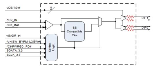
Note: Resistors default to internal on xx42/xx52 devices. P2 devices have programmable default impedances on an output-by-output basis.
