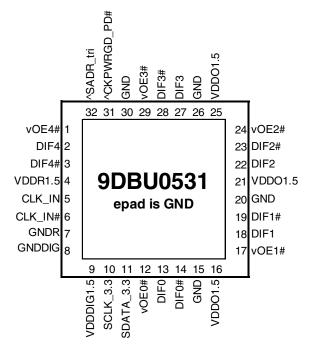
**32-pin VFQFPN, 5x5 mm, 0.5mm pitch** ^ prefix indicates internal 120KOhm pull up resistor
