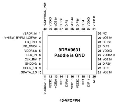
^ prefix indicates internal Pull-Up Resistor
