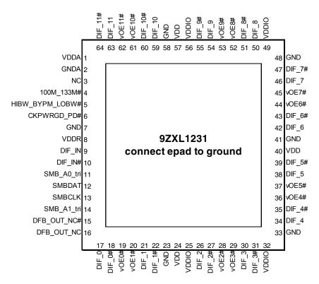
9x9mm 64-pin VFQFPN Note: Pins with ^ prefix have internal 120K pullup Pins with v prefix have internal 120K pulldowm
