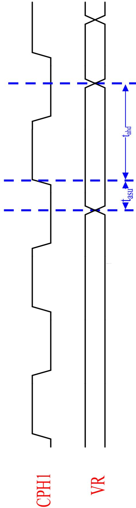
The setup and hold time definition between CPH1 and analog signal VR
