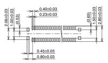
Recommended metal mask pattern Metal mask thickness: When 120µm (Terminal opening ratio: 70%) (Metal-part opening ratio: 100%)
