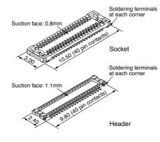
3. Low profile and highly resistant to various environments possible with the use of highly reliable "**TDUGH CONTRET**" connector
