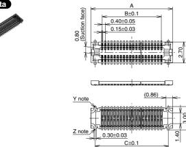
Note: Since the soldering terminals has a single-piece construction, sections Y and Z are electrically connected.
