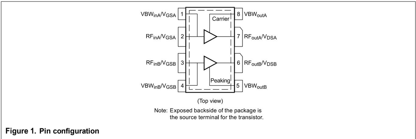
Figure 1. Pin configuration
