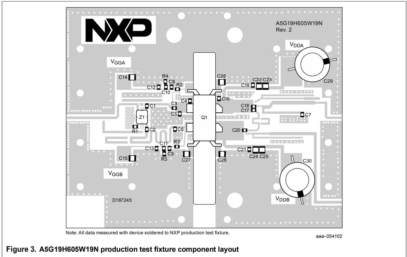
**13.2 Component designations and values****Table 14. A5G19H605W19N production test fixture component designations and values**
