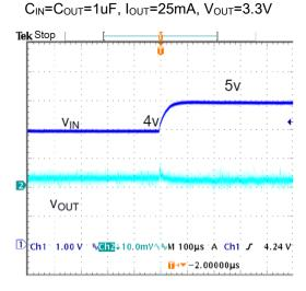
2. Output Voltage vs. Input Voltage
