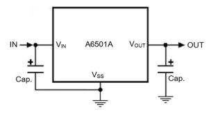
NOTE: Input capacitor ( $C_{IN}$ =1uF) and Output capacitor ( $C_{OUT}$ =3.3uF/4.7uF) are recommended in all application circuit.
