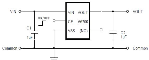
**Caution:** The above connection diagram and constant will not guarantee successful operation. Perform thorough evaluation using the actual application to set the constant.
