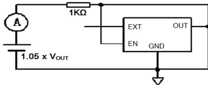
Figure 5. Input Current (no load) test circuit
