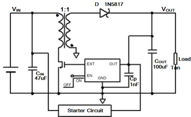
**Note:** In step-down and step-up/step-down application, starter circuit in fig 7 is need. In step-up application, simpler starter circuit in fig 8 can be used.
