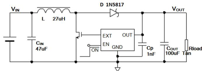
Figure 2. Application with external NPN transistor
