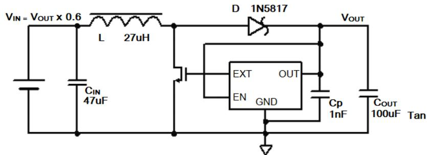
Figure 6. Oscillator frequency and duty cycle test circuit
