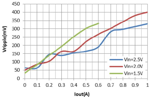
6. Ripple vs. Output Current (5.0V)
