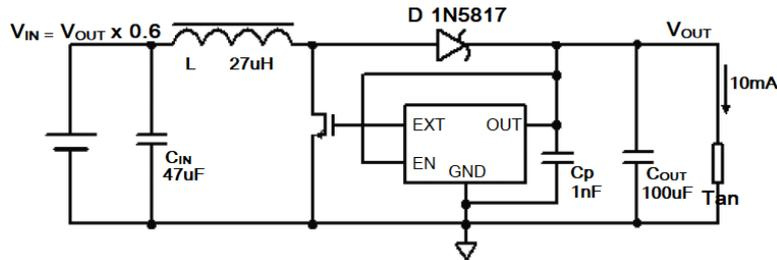
Figure 4. Quiescent current test circuit
