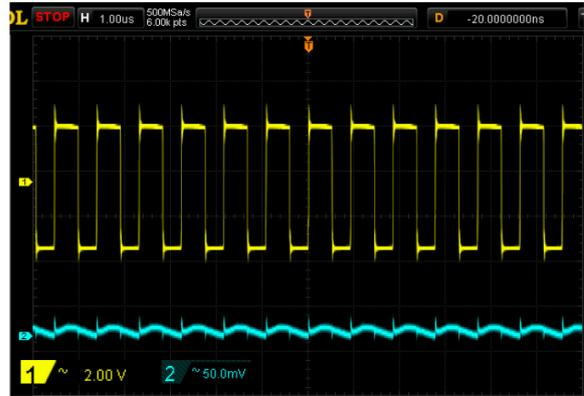
5.  $V_{IN}=3V$ ,  $V_{OUT}=5V$ ,  $I_{OUT}=500mA$ ,
