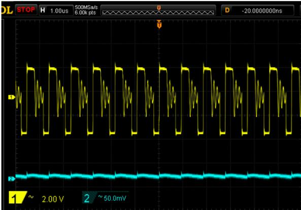
4.  $V_{IN}=3V$ ,  $V_{OUT}=5V$ ,  $I_{OUT}=200mA$ ,
