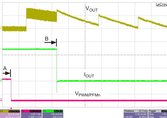
Time A: Transition from PWM to PFM at 250 mA Time B: Load steps from 250 mA to 0 A in Low-IQ PFM mode
