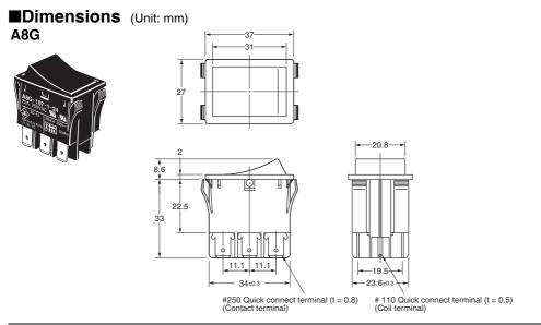
Note: Unless otherwise specified, a tolerance of ±0.8 mm applies to all dimensions.
