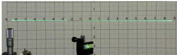
Figure 2. resonant scanning mode on the x-axis (sinusoidal beam motion) used to achieve a large, fast, single-axis resonant axis scan.
