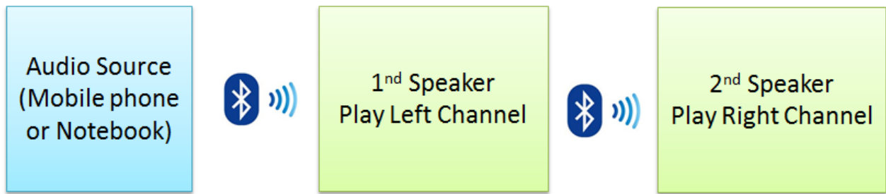
Figure 1-2 AiroStereo Application Block Diagram
