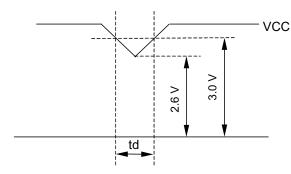
\*2) VCC = +3.3 V, f\_H=37.9 kHz, f\_V=60 Hz, f\_{CLK}=40 MHz
