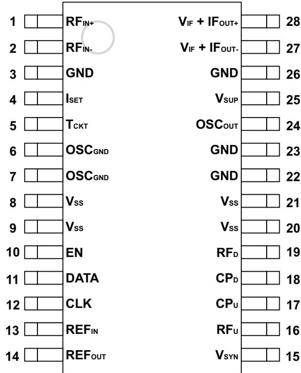
Figure 3: Pinout
