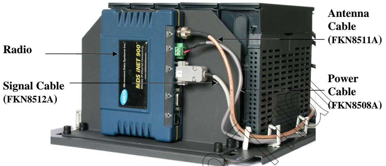
Figure 21-52 iNET 900 Radio Modem Installed on ACE3600 Chassis – Cable Connections
