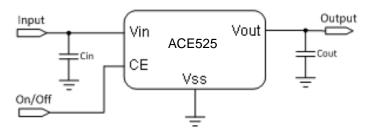
Note: Input capacitor (Cin=1uF) and Output capacitor (Cout=1uF) are recommended in all application circuit.
