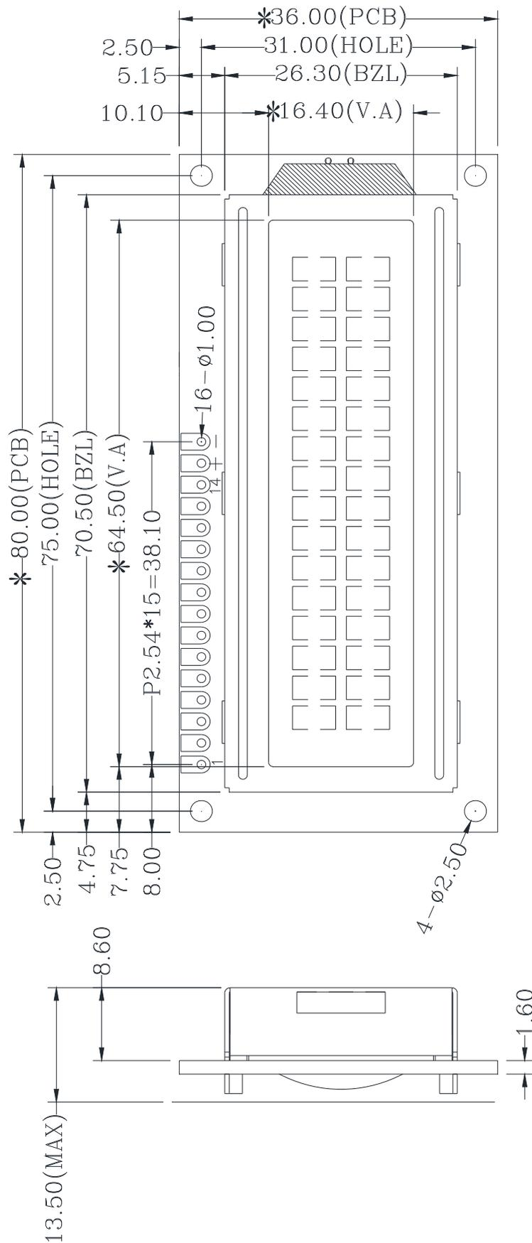
Unspecified tolerance:  $\pm 0.3\text{mm}$
