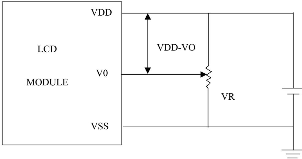
\*  $VDD-V0$  = Operating voltage for LCD
