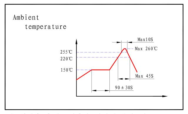
NOTE: After the first reflow, the second reflow is tested on keeping ECM the usual temperature.
