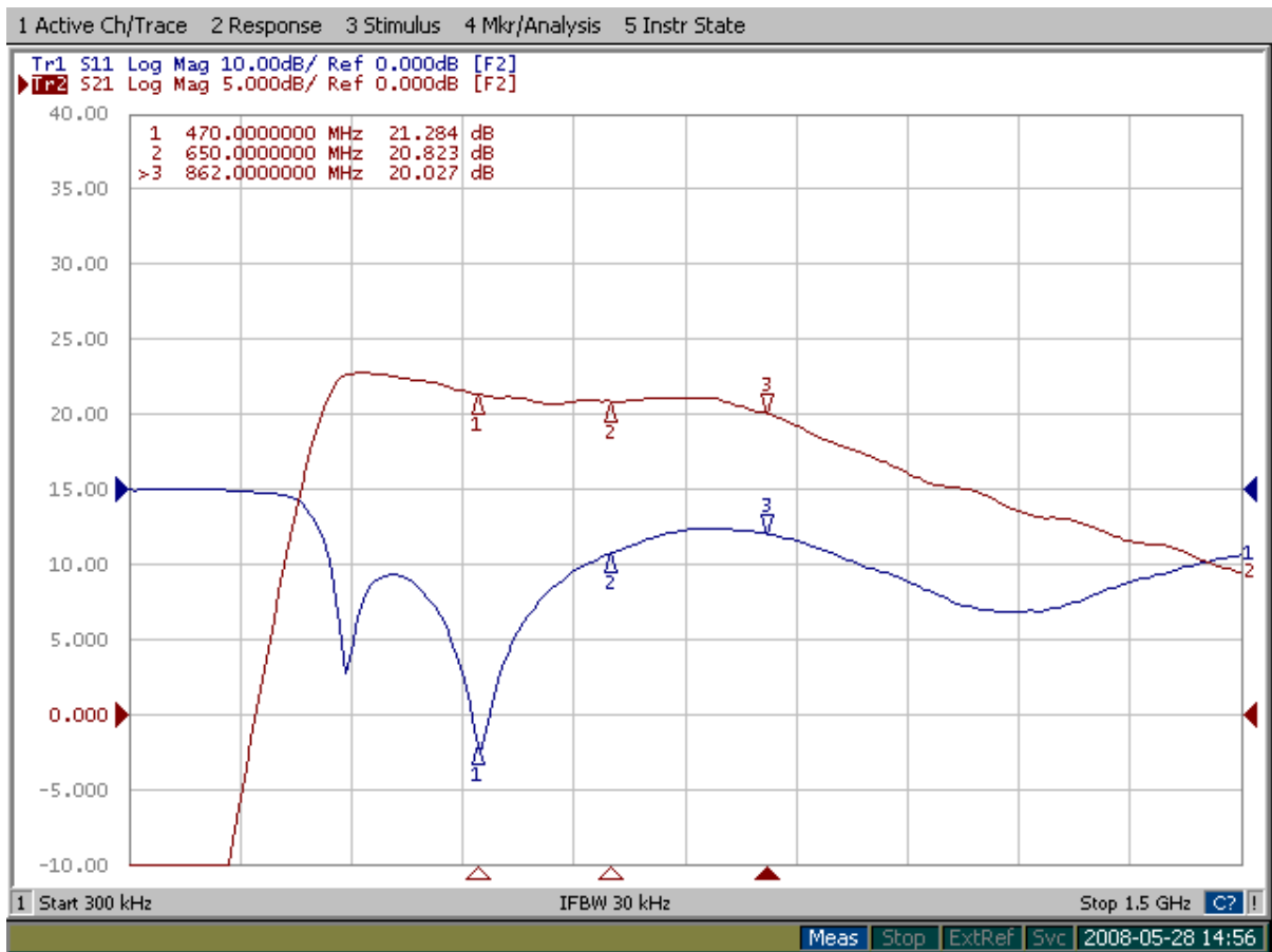
Figure 1: Example of input matching (S11) and transfer function (S21).
