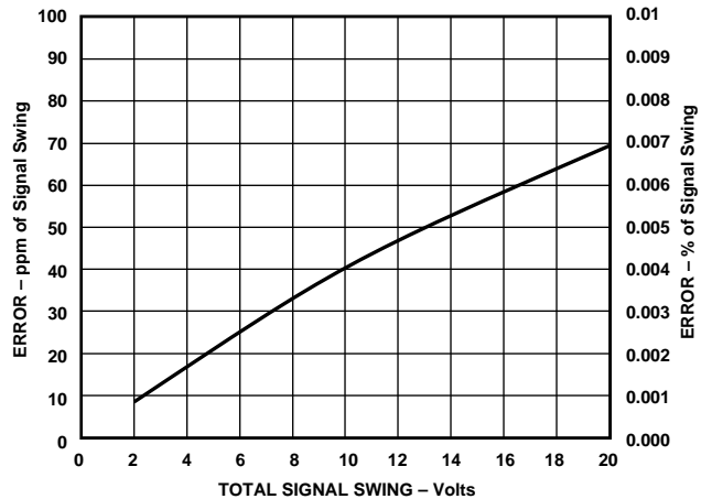
Figure 13. Gain Nonlinearity vs. Output Swing
