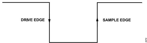
Figure 73. SPI Mode 3, SCLK Edges
