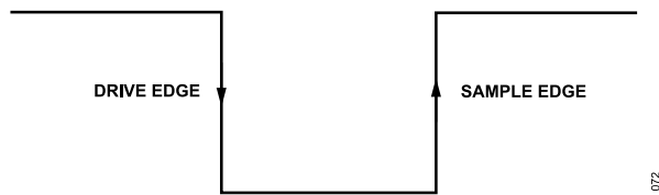
Figure 73. SPI Mode 3, SCLK Edges
