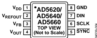
Figure 4. MSOP Pin Configuration
