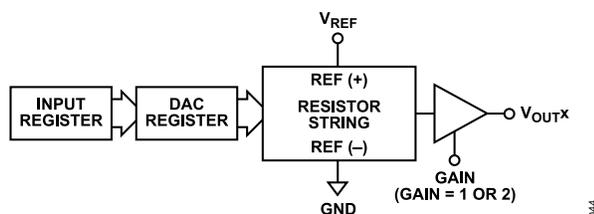
Figure 42. Single DAC Channel Architecture Block Diagram
