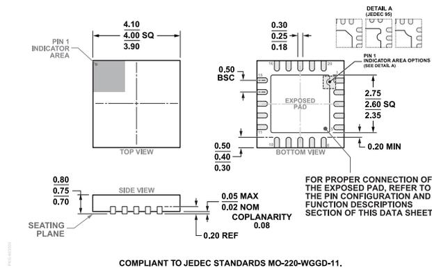
Figure 54. 20-Lead Lead Frame Chip Scale Package [LFCSP] 4 mm x 4 mm Body and 0.75 mm Package Height (CP-20-8)
