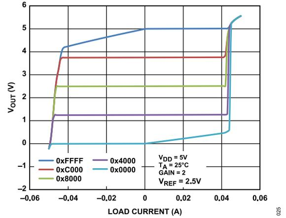
Figure 23. Source and Sink Capability at 5 V
