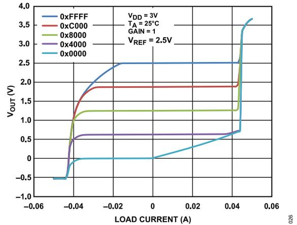
Figure 24. Source and Sink Capability at 3 V
