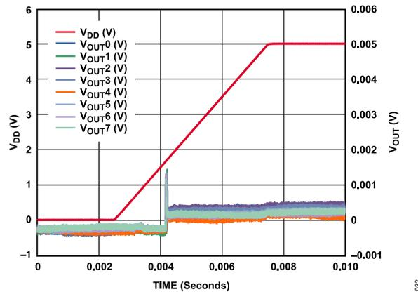
Figure 30. Power-On Reset to 0 V and Midscale
