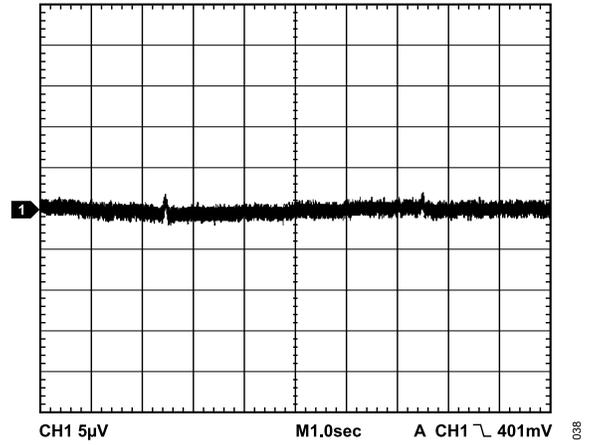
Figure 35. 0.1 Hz to 10 Hz Output Noise
