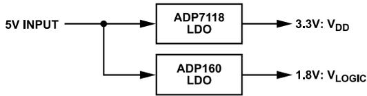
Figure 48. Low Noise Power Solution for the AD5676
