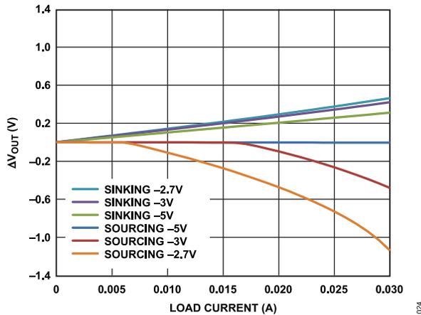
Figure 22. Headroom/Footroom ( $\Delta V_{OUT}$ ) vs. Load Current
