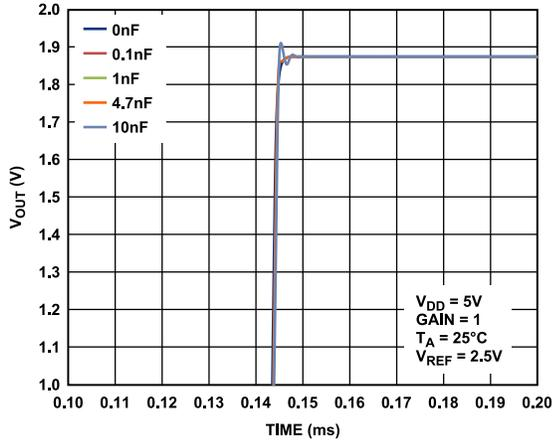
Figure 38. Settling Time for Various Capacitive Loads
