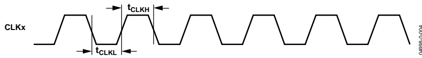
Figure 4. CLK Switching Characteristics (x = A, B, C, D for Individual Input Ports)
