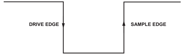
Figure 45. SPI Mode 3 SCLK Edges
