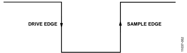
Figure 38. SPI Mode 3 SCLK Edges
