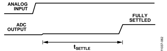
Figure 55. Step Input with Single Cycle Settling
