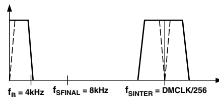
d. Final Filter LPF (HPF) Transfer Function
