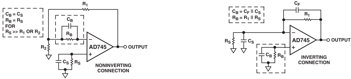
Figure 40. Optional External Components for Balancing Source Impedances
