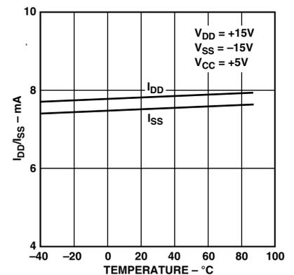
TPC 9.  $I_{DD}$ ,  $I_{SS}$  vs. Temperature
