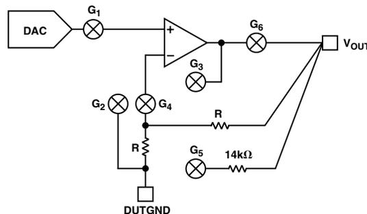
Figure 7. Output Stage After  $\overline{\text{CLR}}$  Is Taken High
