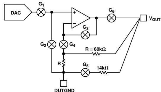
Figure 4. Block Diagram of AD7841 Output Stage
