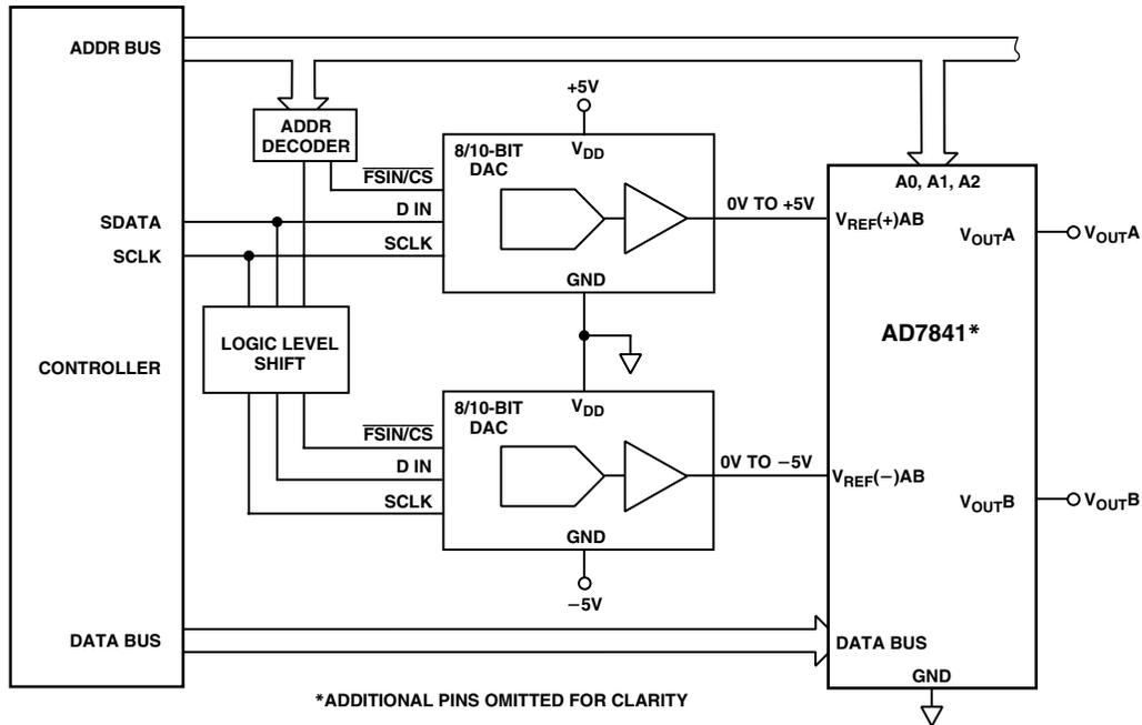
Figure 13. Programmable Reference Generation for the AD7841
