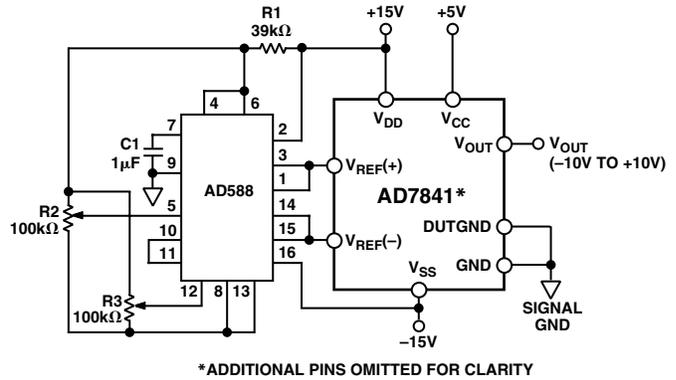
Figure 3. Bipolar  $\pm 10 \text{ V}$  Operation
