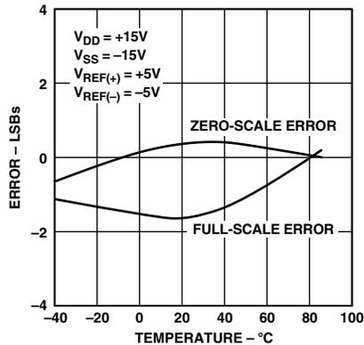
TPC 5. Zero-Scale and Full-Scale Error vs. Temperature
